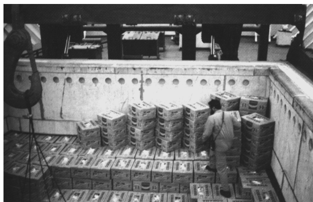
cargo stowed in hatch coamings
